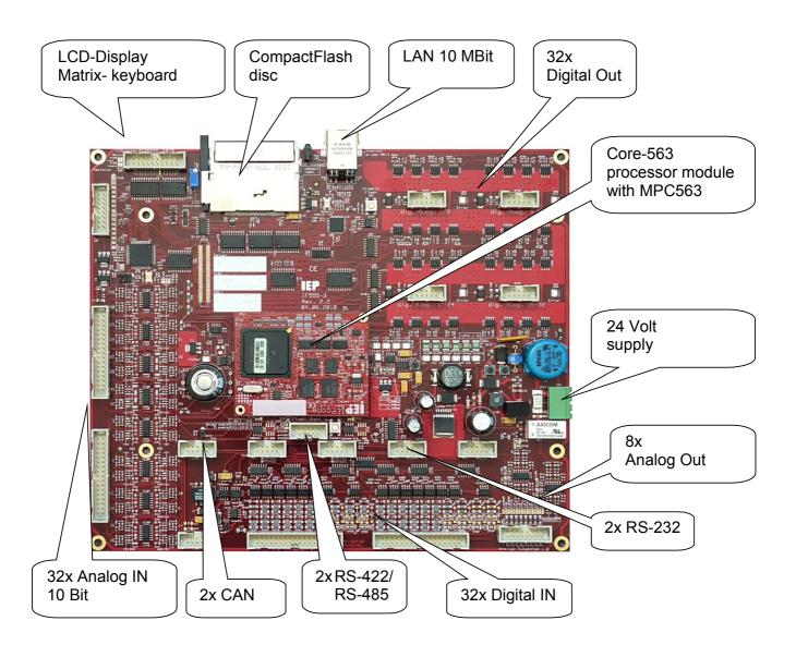
Industrial I/O and high computational power – the **IF555-3** with an automotive PowerPC MPC5xx-Controller, universal I/O and standard interfaces for operating and network is a ready-to-go package for demanding applications in measuring and control engineering.
