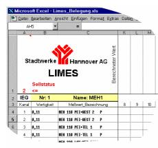
The operating parameters of **LIMES** are configured in Microsoft Excel worksheets on the main computer. The **LIMES** server reads these worksheets on user request and transfers their content to the ZEG. The ZEG stores the parameters locally and distributes them to the IEGs concerned for further local storage.
