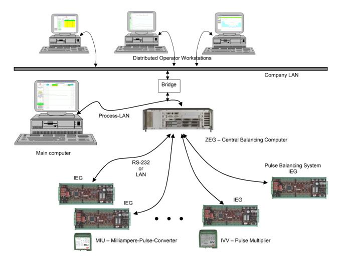
Standard PCs with a Microsoft Windows NT-type operating system and Microsoft Excel can be used as operator workstations. These are connected to the company LAN and use Network-DDE (Dynamic Data Exchange) to access the **LIMES** main computer
