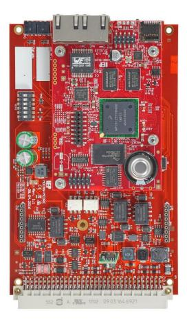
The **MOCAN-M2** is an OEM building block for custom made PLCs and can be used as intelligent subsystem in Ethernet- and CAN-based networks. With up to two independent CAN channels (2.0b), up to 4 serial interfaces as well as digital inputs and outputs, **MOCAN-M2** offers all substantial basic functions of a PLC.
